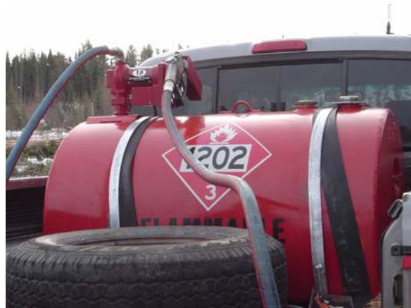
Fuel tanks that adhere to new Transport Canada regulations
