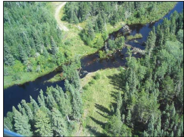
Aerial view of 3-year old rehabilitated Happy Lake Road crossing site, which was removed as part of Tembec road decommissioning.
